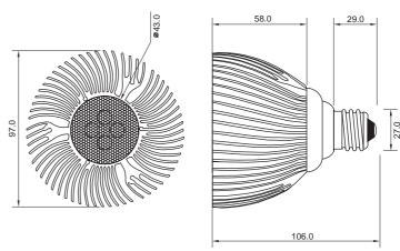
\* The dimensional outline drawings are common in (PAR30-4OWW12W and PAR30-4OWE12W)
